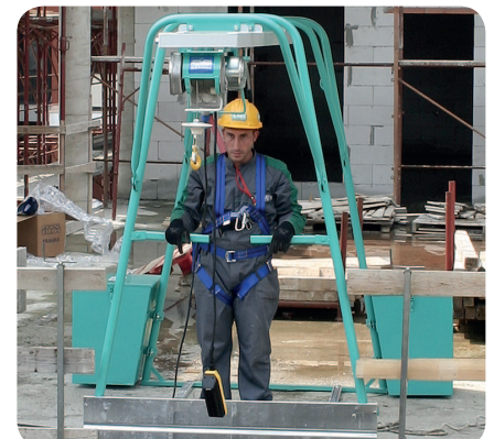
Gantry for stand hoists
